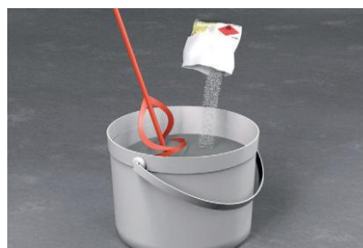
5. Add the catalyst (according to mixing table, temperature and application time) and mix for 2 minutes with a slow-speed stirrer. (Small amounts may also be mixed manually.)
